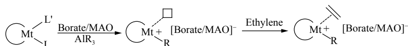
Scheme 1 Formation of cationic active species by metallocene and non-metallocene catalysts (L: ligands)
